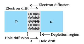
Due to the diffusion of electrons and the holes, from their majority zone to minority zone, a layer of positive and negative space charge region on either side of the junction is formed. This is called the depletion region.
