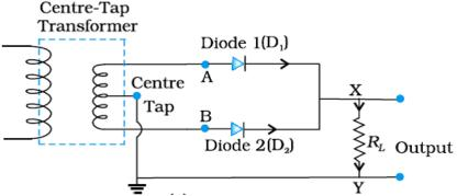
For positive half cycle of input ac, one of the two diodes gets forward biased and conducts and output is obtained across the load R<sub>L</sub>
